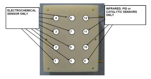
Sensor locations 1 to 8 accommodate the 3-electrode style electrochemical sensors. Locations 5 and 6 will also accommodate electrochemical sensors that require a bias voltage. Locations 7 and 8 will accommodate the typical 3-electrode sensor, and also 2-electrode style electrochemical sensors. (This is typically an oxygen sensor, but some rare gases also fall into this category.)
