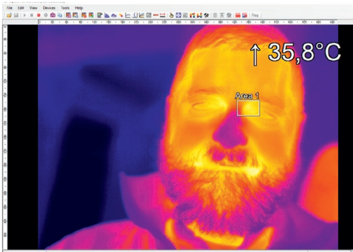
Person coming from inside (exposed for one hour to an ambient of 21 °C)
