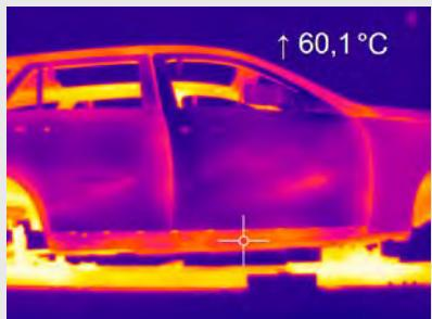
The high-definition optris® PI 640 infrared camera is best used in applications where the very finest thermal details matter.
