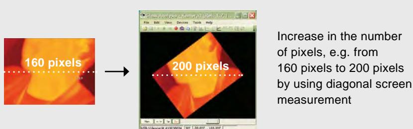
Increase in the number of pixels, e.g. from 160 pixels to 200 pixels by using diagonal screen measurement
