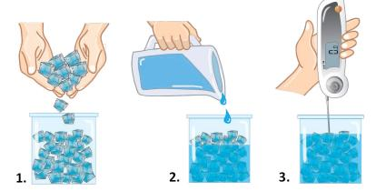
**NOTE:** Instruments without auto hold function - a stable reading for at least 5 seconds must be made. The Testo 104 thermometer probe stabilized reading should display 0°C (±0.5°C). If outside of this range, please return instrument to Eurotec for evaluation
