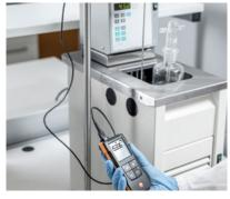
**Temperature:** Digital differential temperature measuring instrument testo 922 gives easy, fast and acurate differential temperature measurement with dual thermocouple Type K probe (2 TC Type K probes included). It has a wide range of applications due to large measuring range from -50 °C to 1000 °C
