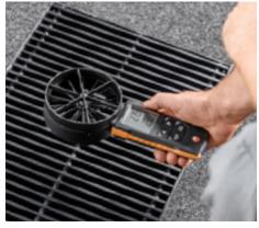
Air Conditioning: You can easily control Air conditioning and ventilation systems with testo flow velocity measuring instruments and ensure that sufficient fresh air is supplied to the rooms and stale air is discharged. You can perform these tasks quickly, easily, precisely and with smart App support: In the duct, at the outlet and when adjusting the balanced residential ventilation.
