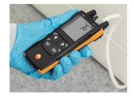
**Pressure:** With the differential pressure measuring instrument testo 512, you can check the gas pressure on burners quickly by measuring gas flow pressure and static gas pressure - indispensable for maintenance work on heating systems. testo 512 is also your reliable partner for general pressure measurement, checking filters and Pitot tube measurement.
