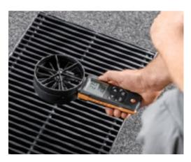
**Air Conditioning:** You can easily control Air conditioning and ventilation systems with testo new flow velocity measuring instruments and ensure that sufficient fresh air is supplied to the rooms and stale air is discharged.
