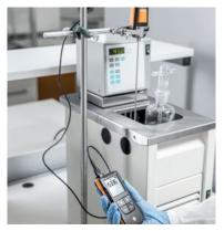
Temperature: Digital differential temperature measuring instrument testo 922 gives easy, fast and precise differential temperature measurement with dual thermocouple Type K probe (2 TC Type K probes included). It has a wide range of applications due to large measuring range from -50 °C to 1000 °C
